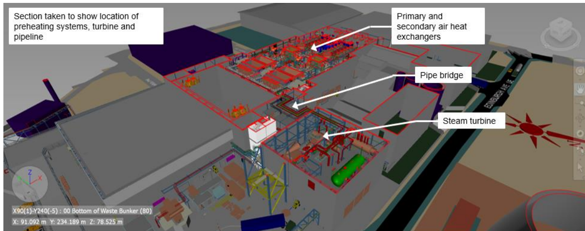
Plate 3.1 – 3D Model Section View of Consented Scheme with external pipework and pipe supports (Note – Proposed Development external pipework is coloured blue)
