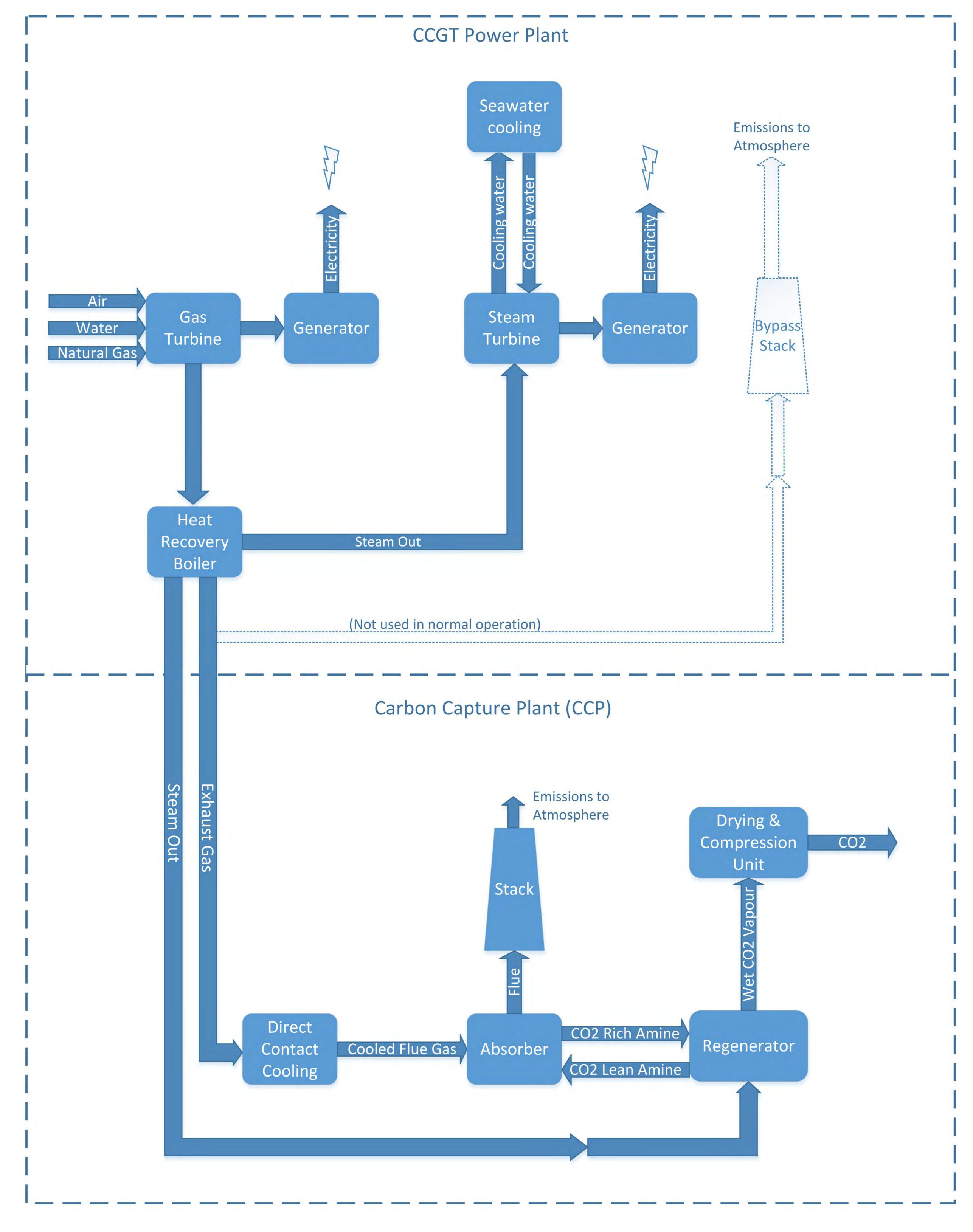
Schematic of CCGT Power Plant and Carbon Capture Plant
