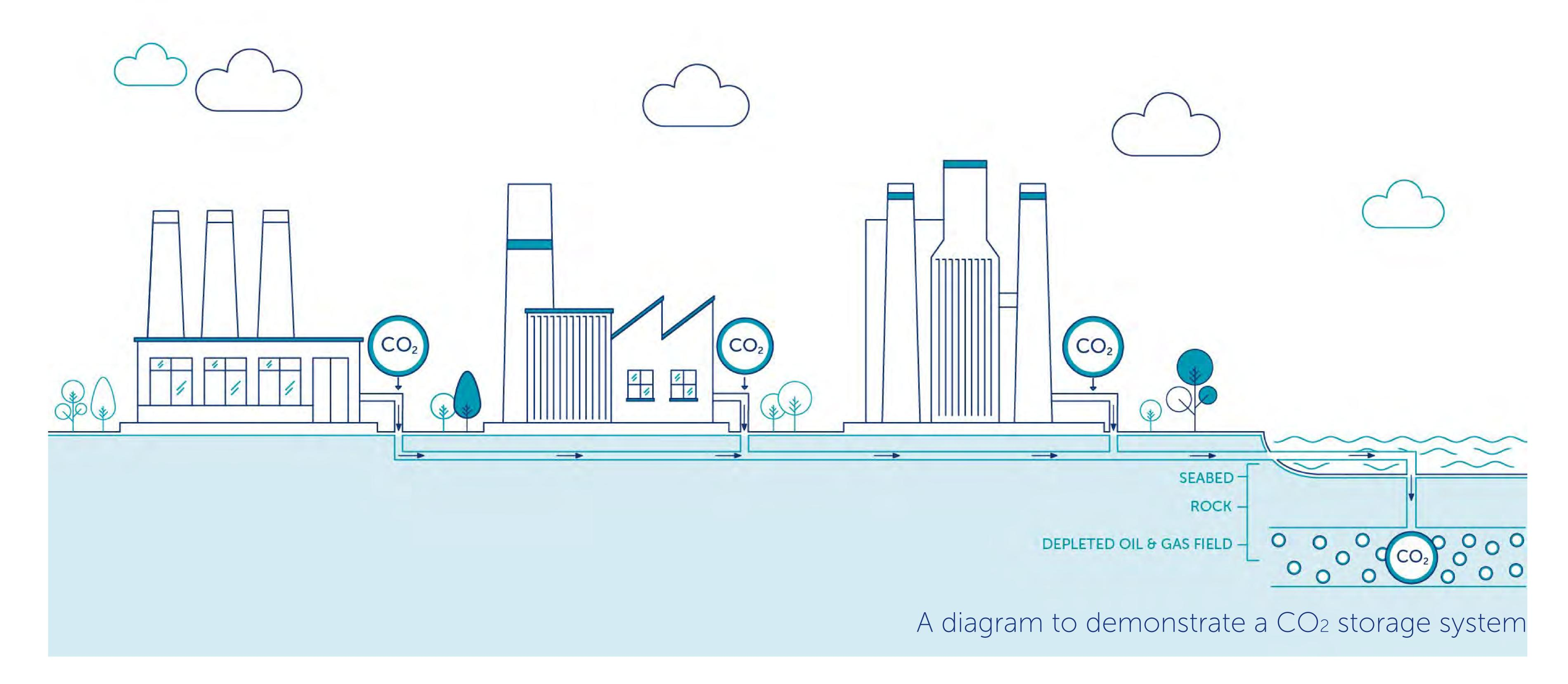
Carbon Capture and Storage (CCS) is a technology that can capture at least 90% of the carbon dioxide (CO<sub>2</sub>) emissions produced from the use of fossil fuels in electricity generation and industrial processes, preventing the CO<sub>2</sub> from entering the atmosphere. The CCS chain consists of three parts; capturing the CO<sub>2</sub>, transporting it, and then securely storing the CO<sub>2</sub> underground, in depleted oil and gas fields or deep saline aquifer formations.
