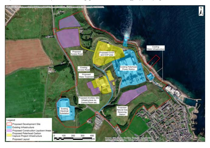
SSE Thermal operates the existing Peterhead Power Station in Aberdeenshire. The Power Station became operational in 1982 and has an output of up to 1,180MW. The Project will be constructed alongside the existing Peterhead Power Station, but with the long-term vision for the Peterhead site to only deliver low-carbon power generation.
